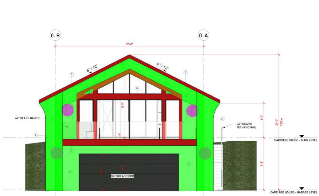
1 CARRIAGE HOUSE - EXTERIOR ELEVATION - ONE SCALE: 1/4" = 1'-0"
