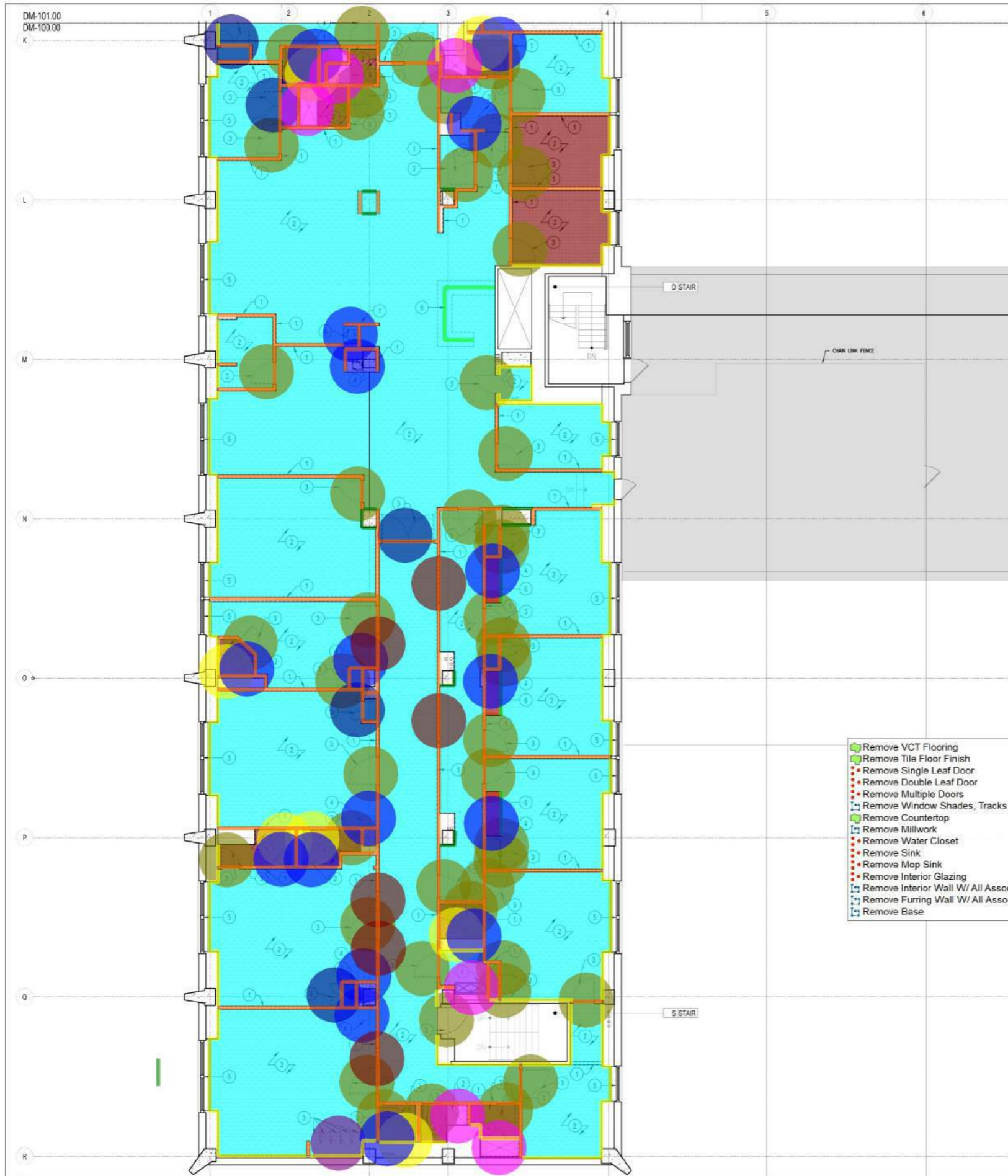
1 | SEVENTH FLOOR DEMOLITION PLAN
